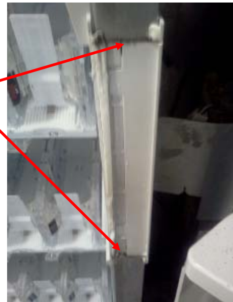
Remove bowed metal from the Delivery Door area as shown.
