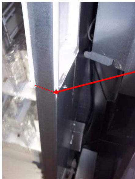
Remove bowed metal from the Delivery Door area as shown.
